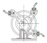
According to each mounting application, recommend Guide Arm positions. Replace and tighten the nuts and washer.
